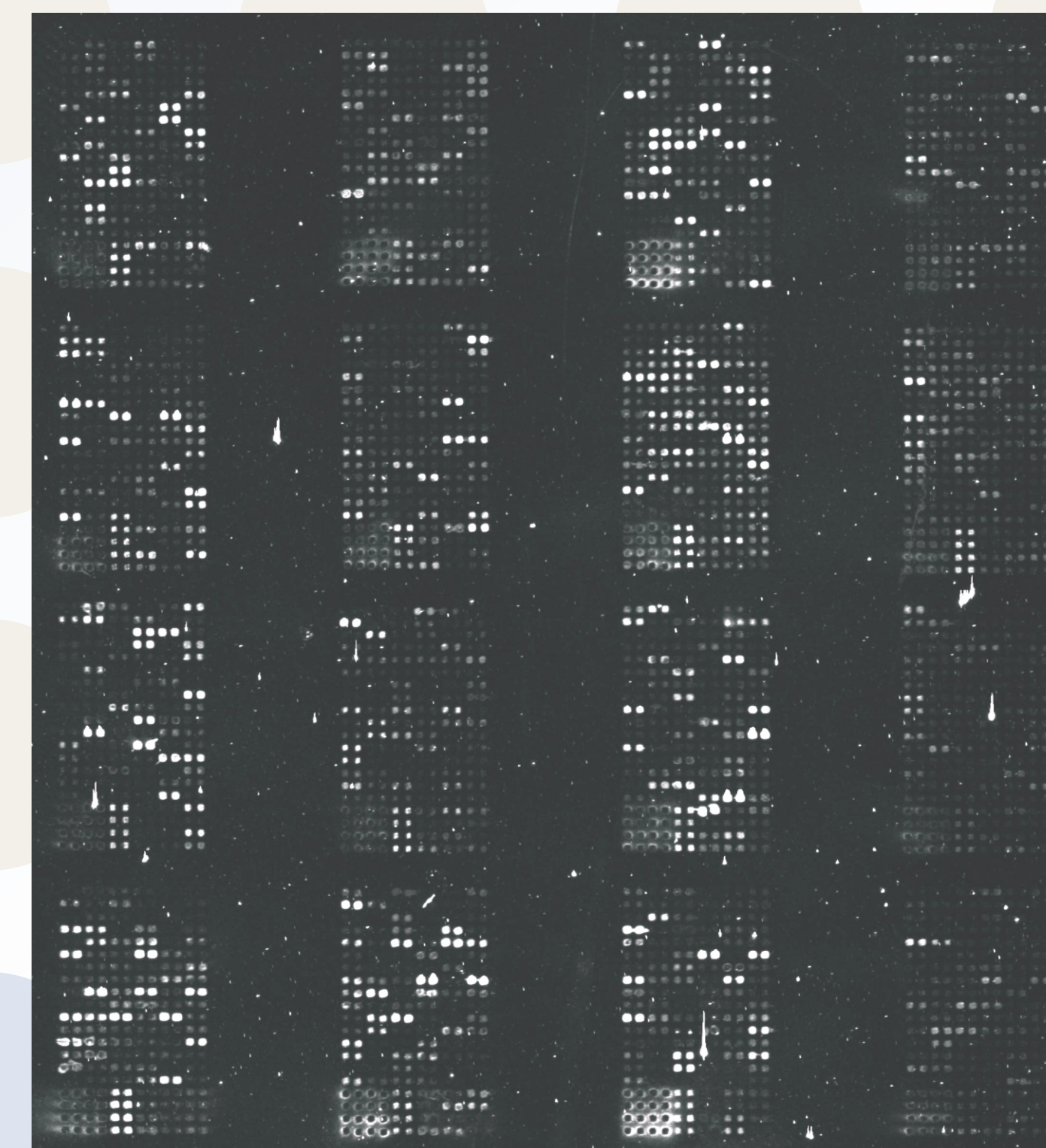
Figure 3. A Hum1.7k4 array hybridized with biotin-labelled cDNA made from 2 µg of Human Universal Reference RNA (Stratagene). The exposure time for this image is 1 second. The image obtained from the Au RLS Particles™ is shown.
